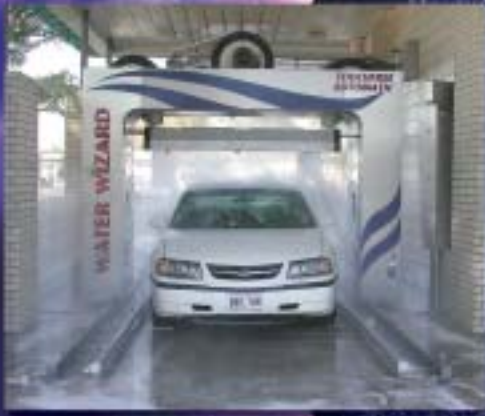
The entire vehicle will receive a good scrubbing as the high pressure water creates friction upon impact with the vehicle's surface.
