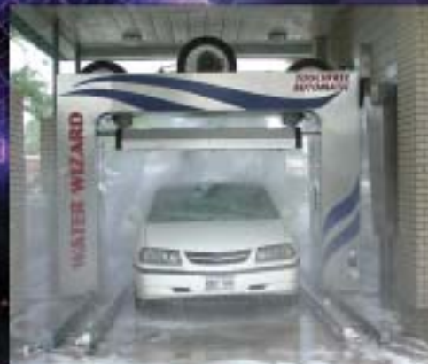
The scrubbing, oscillating nozzles sweep back and forth as the wash gantry passes over the vehicle.
